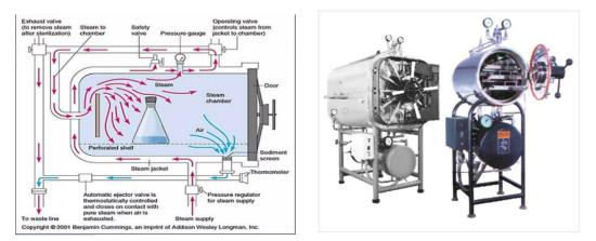
**Figure:** Diagrammatic Representation and photos of Rectangular and cylindrical Horizontal Double Jacketed Autoclave
